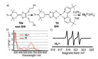
Fig. 8 (a) Molecular structures of radical ligand tempodt 10a, platinum–tempodt complex 10, with the formation of the dimerized complex  $10_2^{2+}$  and (b) the UV-vis spectra of 10 and  $10_2^{2+}$ ; (c) EPR spectrum of  $10_2^{2+}$ . Figures adapted with permission from ref. 106. Copyright 2008 American Chemical Society.
