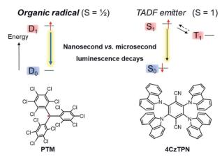
Fig. 2 Comparison of the emission process of the organic radical emitter *per*-chlorotriphenylmethyl PTM (left) and the TADF emitter 2,3,5,6-tetra(9*H*-carbazol-9-yl)terephthalonitrile, **4CzTPN** (right).<sup>44</sup>
