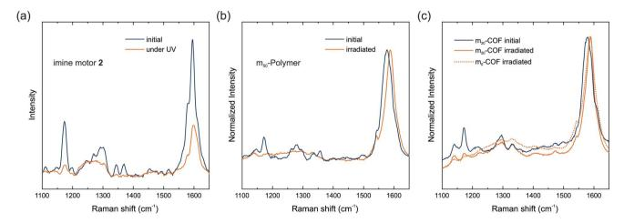
Fig. 4 Raman spectra of the imine motor 2 as a thin-film (a),  $m_{50}$ -P (b), and  $m_{20}$ -COF. The thin-film of the molecular imine motor 2 was recorded at 785 nm and irradiated at 365 nm with a UV-LED. Raman spectra of  $m_{50}$ -P (b),  $m_{20}$ -COF and  $m_{0}$ -COF (c) were recorded with a Raman laser at 355 nm for simultaneous excitation of the motor.
