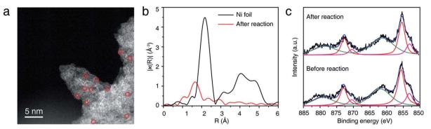
Fig. 3 (a) Representative HAADF-STEM image, (b) Ni K-edge EXAFS spectra, and (c) XPS spectra of NiSAC/CN after the model reaction.
