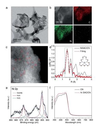
Fig. 1 (a) Representative TEM image, (b) EDS mapping image, (c) HAADF-STEM image, (d) Fourier transform of Ni K-edge EXAFS spectra (silver: Ni, grey: N, brown: C), and (e) Ni 2p XPS spectra of NiSAC/CN. (f) UV-vis spectra of CN and NiSAC/CN.
