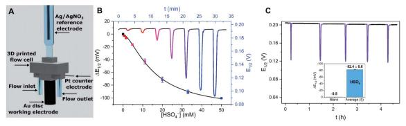
Fig. 30 (A) Schematic depiction of the 3D-printed electrochemical flow cell. (B) Sensogram (blue axes) and corresponding isotherm (black axes) of  $28.XB_{SAM}$  under continuous flow to increasing concentrations of  $HSO_4$  in  $HSO_4$  additions. Reproduced from ref. 72 under the terms of the  $HSO_4$  increase.
