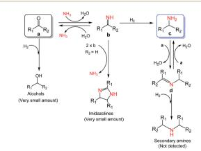
Fig. 5 Proposed mechanism for the reductive amination of carbonyl compounds to primary amines using  $NH_3$  and  $H_2$  over Co@C-N(800).
