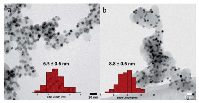
Fig. 1 TEM micrographs of (a) binary oh-PtNi and (b) oh-PtNi(RhMo); the insets show the corresponding mean edge-length size distribution histogram.
