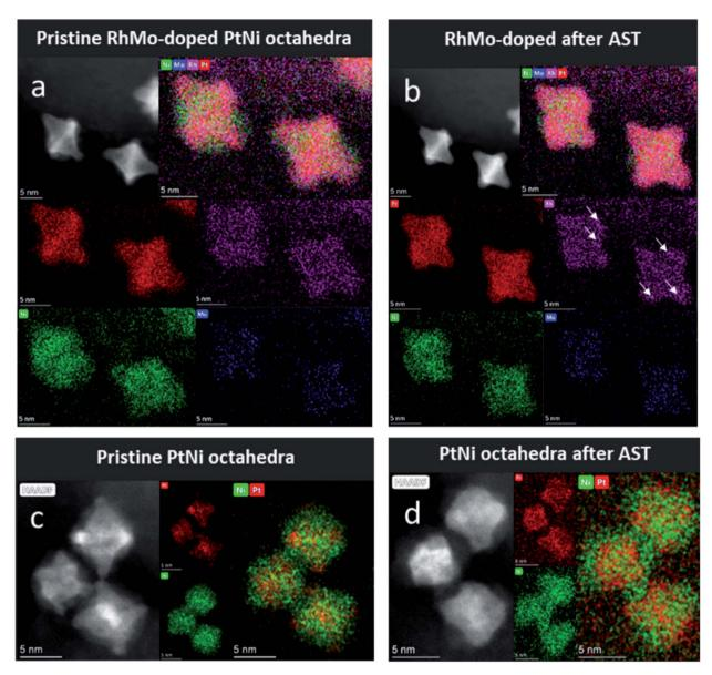
Fig. 3 IL-HAADF-STEM images (grey) and STEM-EDX composition maps of the pristine state (a) and (c) and after an AST of 10 800 cycles between 0.6 and 0.95  $V_{RHE}$  at a scan rate 1 V s<sup>-1</sup> (b) and (d) for RhMo-doped PtNi (Pt in red, Ni in green, Rh in purple, and Mo in blue) and PtNi octahedra.
