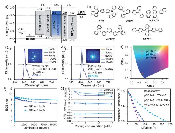
Fig. 3 (a) Device configuration with an energy-level diagram and (b) the molecular structures of the materials used in this device. (c and d) The EL spectra of the devices, and (e) EQE versus luminance curves of devices A1 and B1. (f) Luminescence and current density versus voltage. (g) The EQE<sub>max</sub>, FWHMs and CIE<sub>y</sub>-dopant concentration relationships in devices. (h) The device luminance versus lifetime curves measured at 2000 cd
