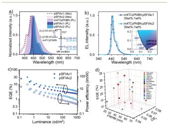
Fig. 4 (a) The absorption spectra of MR emitters and the PL spectra of the doped films of mCBP: 30 wt% m4TCzPhBN; mCBP: 30 wt% m4TCzPhBN: 1 wt% MR emitters. (b) The EL spectra of devices were recorded at 1000 cd m<sup>-2</sup>. (c) The EQE and PE versus luminance curves of the devices. (d) Summary of the EQE versus FWHMs and CIE, color coordinates plot of deep-blue materials reported in the literature. The red star represents the results of the present work.
