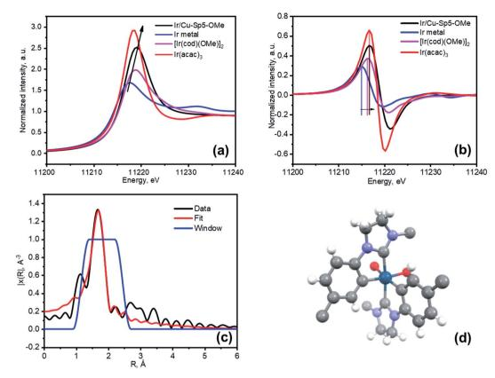
Fig. 4 (a) XANES spectra of Ir/Cu-Sp5-OMe compared to Ir metal,  $[Ir(cod)(OMe)_2]$  and  $Ir(acac)_3$  references, (b) First derivative of the XANES spectra from (a) and (c) Fitted EXAFS spectrum of Ir/Cu-Sp5-OMe in R-space (d) A model of iridium arrangement in Ir/Cu-Sp5-OMe. Atom colors: Ir, dark blue; C, grey; C, red; C, blue; C, white. The C-bracket is expected that the two additional coordination sites on the C-bracket is likely to be two THF molecules.
