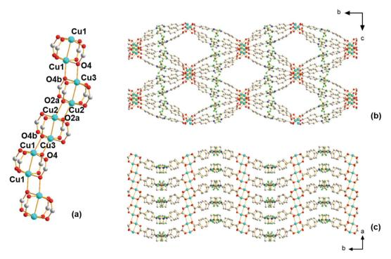
Fig. 2 Structure of Cu-Sp5-BF<sub>4</sub>-A. (a) View of SBU, (b) view along the a axis depicting channel front, and (c) view along the c axis depicting walls of the channel and paddlewheel SBUs. Hydrogen atoms are omitted for clarity. Atom colors: C, gray; O, red; N, blue; H, white; B, brown; F, green; Cu, turquoise.
