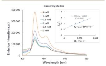
Fig. 3 Luminescence quenching studies. Stern–Volmer plot (inset) of the intramolecular cyclization of **3b**.
