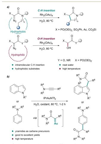
Fig. 4 C-H insertion reactions in water. (a) Intramolecular insertion of rhodium carbenoids into aliphatic C-H bonds reported by Afonso and coworkers. (b) Functionalization of indoles and anilines by *in situ* generated  $\alpha$ -oxo gold carbenes.
