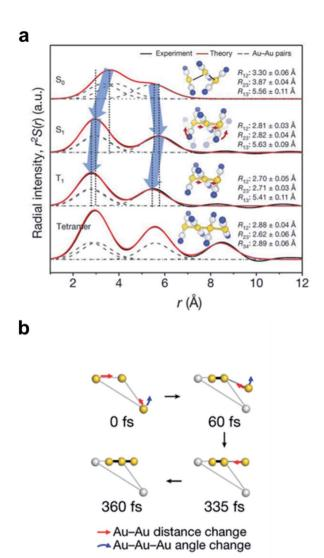
Fig. 2 (a) Radial distribution functions of the four states of [Au(CN)<sub>2</sub><sup>-</sup>]<sub>3</sub> determined from a fs-TRXL study. Reproduced from ref. 62 with the permission of Springer Nature, copyright 2015. (b) The transient structures associated with the bond-formation dynamics at representative time delays. Reproduced from ref. 63 with the permission of Springer Nature, copyright 2020
