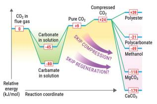
Fig. 3 Conceptual energy comparison for capture and conversion of  ${\rm CO}_2$ .
