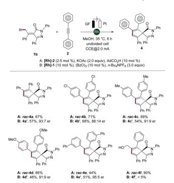
$\begin{array}{lll} \textbf{Scheme 4} & \textbf{Enantio-selective rhoda-electrocatalyzed spiroannulation} \\ \textbf{of pyrazolone 1b}. \end{array}$
