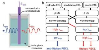
**Fig. 6** (a) Scheme showing light conversion by PECL. (b) Scheme showing the possible combinations of ECL systems and SCs, leading to the two PECL categories.
