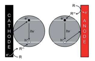
Scheme 1 ECL promotion with QDs. The e<sup>-</sup>/h<sup>+</sup> pairs are injected separately by the electrode and the co-reactant, respectively following either the cathodic (left) or anodic ECL pathway (right). Adapted from ref. 181 with permission from the American Chemical Society, Copyright 2014.
