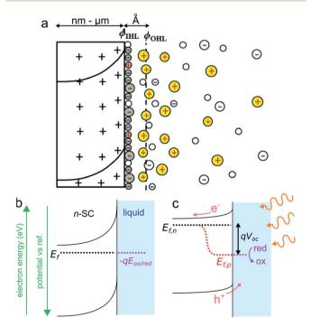
Fig. 3 (a) Scheme of the space charge layer in an n-SC (left) and the Helmholtz layer at the SC/liquid interface (right), adapted with permission from ref. 92  $\phi_{IHL}$  and  $\phi_{OHL}$  are the inner and the outer Helmholtz planes. (b) Scheme showing a depleted n-SC in equilibrium with an electrolyte containing the ox/red redox couple in the dark. (b) Scheme showing the effect of illumination  $(h\nu > E_a)$  on this junction.
