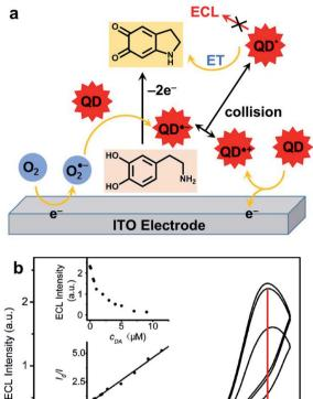
Fig. 10 Detection of catechol with CdTe QDs. (a) Chemical mechanism leading to ECL quenching. (b) ECL curves collected in phosphate
