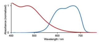
Fig. 10 Solid-state absorption spectra of  $FTO/TiO_2$  electrodes with adsorbed dyes  $[Cu(11)(45)]^+$  (red) and SQ2 (blue). The high-energy tail arises from  $TiO_2$  absorption (spectra recorded by Frederik Malzner, University of Basel).
