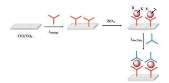
Fig. 15 The SALSAC approach to *in situ* assembly of a heteroleptic bis(terpyridine)zinc( $\pi$ ) dye on an electrode surface using a stepwise strategy. ZnX<sub>2</sub> is typically Zn(OAc)<sub>2</sub> or ZnCl<sub>2</sub>.
