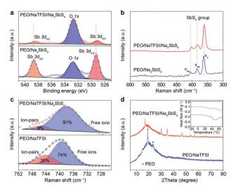
Fig. 3 Interactions between components in the PEO-based all-solidstate electrolytes. (a) Sb 3d XPS spectra and (b) Raman spectra of the PEO/Na<sub>3</sub>SbS<sub>4</sub> and PEO/NaTFSI/Na<sub>3</sub>SbS<sub>4</sub> electrolyte. (c) Raman spectra and (d) XRD patterns of the PEO/NaTFSI electrolyte and PEO/NaTFSI/ Na<sub>3</sub>SbS<sub>4</sub> electrolyte. Inset: corresponding DSC curves.
