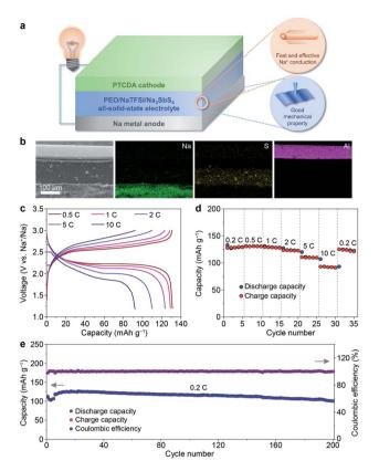
**Fig. 6** Characterization and performance of all-solid-state Na–PTCDA batteries. (a) Schematic illustration, (b) cross-sectional SEM image and corresponding elemental mappings of the battery. (c) Discharge/charge profiles, (d) rate performance at different current rates, and (e) cycling performance at 0.2C (the rates of the initial 5 cycles were set as 0.1C for activation) of the batteries (45 °C).
