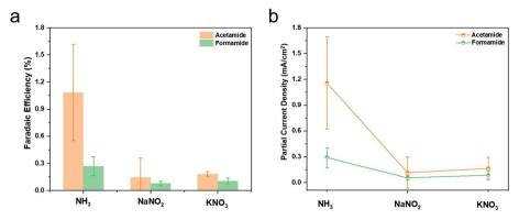
Fig. 5 In the equivalent reaction setup as in Fig. 3 with Cu catalysts and  $NO_2^-$  (0.5 M) or  $NO_3^-$  (1 M) in place of  $NH_3$  at -0.98 V vs. RHE, formamide and acetamide were generated. The faradaic efficiencies (a) and partial current densities (b) for their generation were compared to those from using NH<sub>3</sub>.
