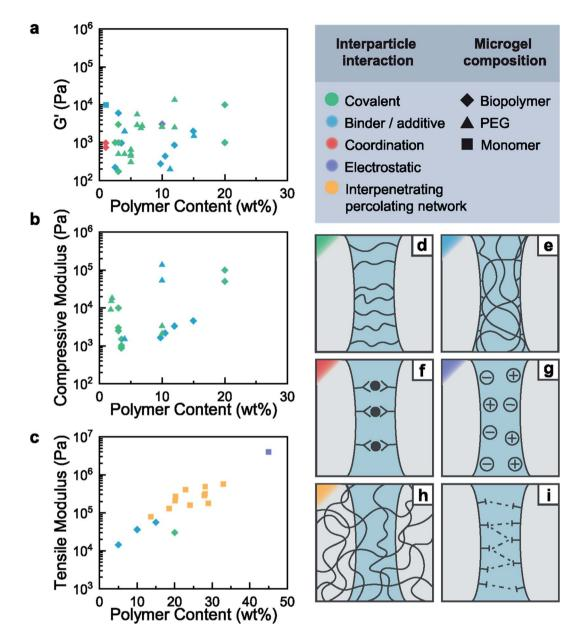
Fig. 2 Elastic mechanical properties of granular hydrogels cured through various interparticle binding strategies. Ashby plots of the storage (a), compressive (b), and tensile (c) modulus as a function of polymer content. Schematic representation of the interparticle interaction mechanisms: covalent interaction (d), binder and additives (e), coordination interactions (f), charge interactions (g), interpenetrating percolating network (h) and other supramolecular interactions (i).
