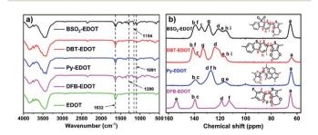
Fig. 1  $\,$  (a) FT-IR spectra and (b) solid-state  $^{13}\mathrm{C}$  NMR spectra of the asprepared CPs.
