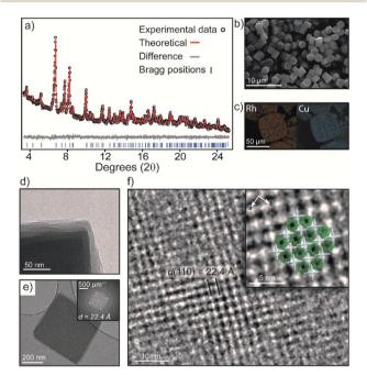
Fig. 3 (a) Rietveld refinement of the PXRD data of 3; (b) SEM image of 3 obtained from a DMF recrystallization; (c) EDX elemental mapping of Cu and Rh within crystals of 3; TEM images of 3 (d) the edge of a crystal, showing misalignment of layers; (e) the FFT pattern of a selected crystal; (f) an enlarged image of the same crystal showing the superimposition of the crystal structure of 3 along the c axis.
