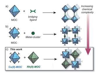
Fig. 1 Strategies to synthesise MOFs from preformed MOCs; (a) utilising bridging ligands to link MOCs via the available coordination sites;<sup>23</sup> (b) linking surface-functionalised MOCs via a metal cluster;<sup>24</sup> (c) this work: linking a surface-functionalised Cu(II) MOC to a Rh(II) MOC via preferential Rh-aniline coordination.
