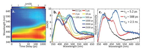
Fig. 3 (a) TA spectra of 1.1 mM AQS in 0.1 M acetate buffer pH 4.9, 0.2 M KCl represented as a false colour map showing changes in optical density ( $\Delta$ mOD) with photoexcitation at 330 nm; (b) different time delays ( $\Delta t$ ) chosen for the TA spectra; (c) the corresponding evolution-associated difference spectra (EADS) from the global fit.
