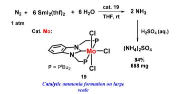
Fig. 22 Molybdenum-catalysed nitrogen fixation using samarium diiodide with water.
