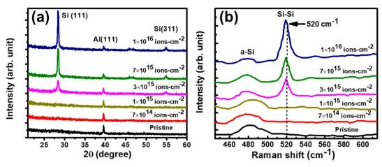
Fig. 10 (a) XRD pattern (b) Raman spectra of pristine sample and the samples irradiated with different ion fluence of  $7 \times 10^{14}$  ions per cm<sup>2</sup>,  $1 \times 10^{15}$  ions per cm<sup>2</sup>,  $3 \times 10^{15}$  ions per cm<sup>2</sup>,  $7 \times 10^{15}$ , and  $1 \times 10^{16}$  ions per cm<sup>2</sup>. [Reproduced/adapted from Maity *et al.*, <sup>161</sup> *J. Appl. Phys.*, 2022, **132**, 095303, with the permission from AIP Publishing.]
