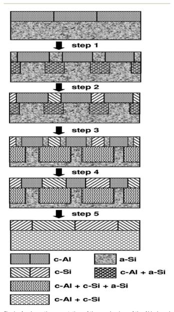
Fig. 1 A schematic presentation of the mechanism of the Al induced layer exchange process. [Reproduced/adapted from Wang et al., <sup>16</sup> J. Appl. Phys., 2007, **102**, 113523, with the permission from AIP Publishing.]
