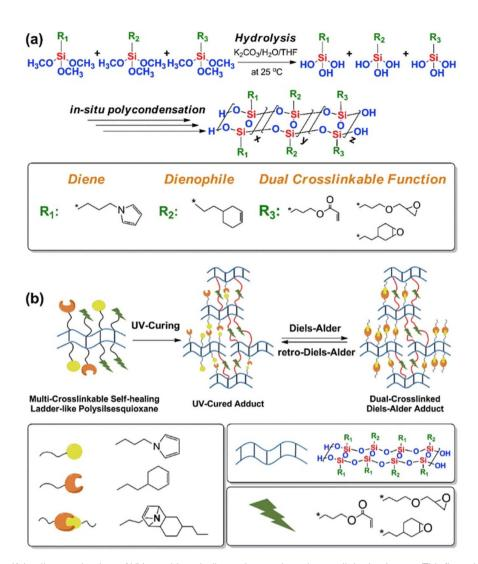
Fig. 3 Synthesis and self-healing mechanism of UV-curable polysilsesquioxane-based cross-linked polymers. This figure has been adapted from ref. 33 with permission from Elsevier, copyright 2017.
