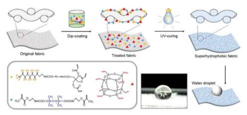
Fig. 12 Preparation of UV curable superhydrophobic self-healing textile coating. This figure has been adapted from ref. 58 with permission from Elsevier, copyright 2017.
