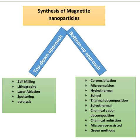
Fig. 4 Techniques to synthesize magnetite nanoparticles.
