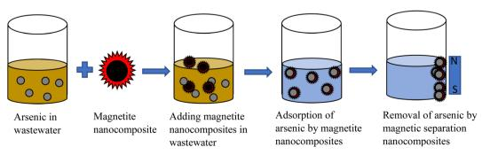
Fig. 3 Process of arsenic removal from wastewater using magnetite nanocomposites.
