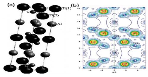
Fig. 2 (a) Crystal assembly and (b) charge density distribution pattern of Ti<sub>3</sub>AlC<sub>2</sub>.<sup>25</sup>
