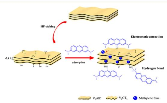
Fig. 10 Mechanism of adsorption of MB on V<sub>2</sub>CTx MXene surface. 117
