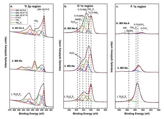
Fig. 5 XPS spectra with curve-fitting for (a) Ti 2p region for (i) Ti<sub>3</sub>C<sub>2</sub>T<sub>x</sub>, (ii) MX-Na (iii) MX-Na-A. (b) O 1s region for (i) Ti<sub>3</sub>C<sub>2</sub>T<sub>x</sub>, (ii) MX-Na (iii) MX-Na-A. (c) F 1s region for (i) Ti<sub>3</sub>C<sub>2</sub>T<sub>x</sub>, (iii) MX-Na-A. (iii) MX-Na-A.
