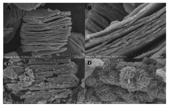
Fig. 8 SEM images of pure Ti<sub>3</sub>C<sub>2</sub> (A and B) and MoS<sub>2</sub>-Ti<sub>3</sub>C<sub>2</sub> (C and D).<sup>95</sup>
