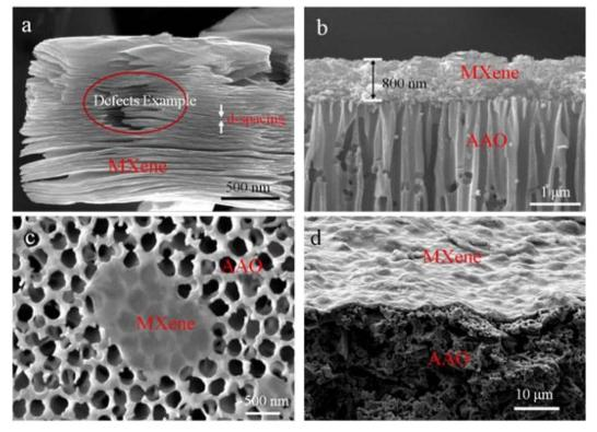
Fig. 4 (a and b) SEM images of cross-section of Ti<sub>3</sub>C<sub>2</sub>T<sub>x</sub> (c) Top view and (d) low magnification cross section.<sup>47</sup>
