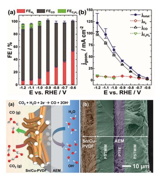
Fig. 2 (Up): (a) Faradaic efficiencies, (b) current densities for electrochemical  $CO_2$  reduction at a Sn/Cu-PVDF GDE at (-0.6 to -1.2 V vs. RHE). (Bottom): (a) Scheme and (b) cross-sectional SEM image of a Sn/Cu-PVDF/AEM assembly used for electrocatalytic reduction of gaseous  $CO_2$ . Reproduced with permission.<sup>66</sup> Copyright ©2019, Wiley-VCH.
