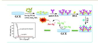
Fig. 3 Schematic diagram of ultra-sensitive detection of CEA by immunosensor. Reproduced from ref. 33 with permission from Royal Society of Chemistry.
