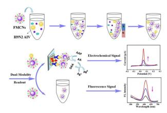
Fig. 5 Schematic diagram of fluorescence and electrochemical dualmode immunoassay platform for detection of avian influenza virus. Reproduced from ref. 39 with permission from American Chemical Society.
