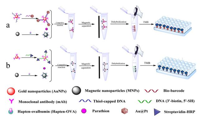
Fig. 8 Schematic presentation of the colorimetric Bio-Barcode Immunoassays using (a) Au@Pt and (b) HRP amplification. Reproduced from ref. 60 with permission from American Chemical Society.
