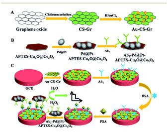
Fig. 2 Schematic diagram of the principle of electrochemical immunosensor for PSA detection based on multi-signal amplification. Reproduced from ref. 25 with permission from Royal Society of Chemistry.
