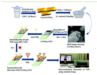
Fig. 7 Schematic diagram of electrochemical immunosensing platform for NSE detection based on CS/MoS<sub>2</sub>. Reproduced from ref. 55 with permission from Royal Society of Chemistry.
