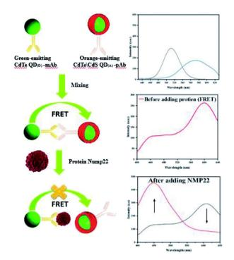
Fig. 13 Schematic diagram of NMP22 detection using fluorescence immunosensing platform based on two different semiconductor quantum dots. Reproduced from ref. 87 with permission from Royal Society of Chemistry.
