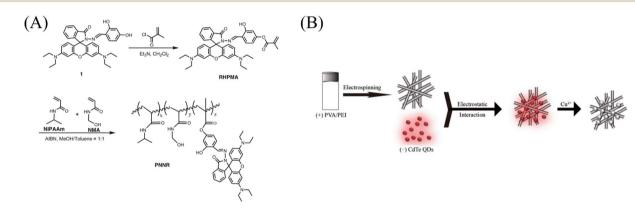
Fig. 5 Preparation of copper ion sensor by copolymerization and surface adsorption and their sensing mechanism. (A) Reprinted with permission from ref. 90. Copyright 2016, Springer Science Business Media Dordrecht. (B) Reprinted with permission from ref. 91. Copyright 2021 Changchun Institute of Applied Chemistry, Chinese Academy of Sciences. Published by Elsevier.
