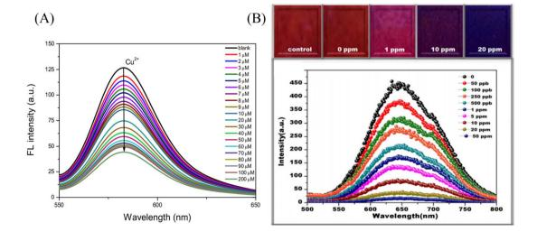
Fig. 6 Sensing properties of copper ion sensors preparted by copolymerization and surface adsorption. (A) Reprinted with permission from ref. 90. Copyright 2016, Springer Science Business Media Dordrecht. (B) Reprinted with permission from ref. 92. Copyright 2015, Senthamizhan, A. et al.
