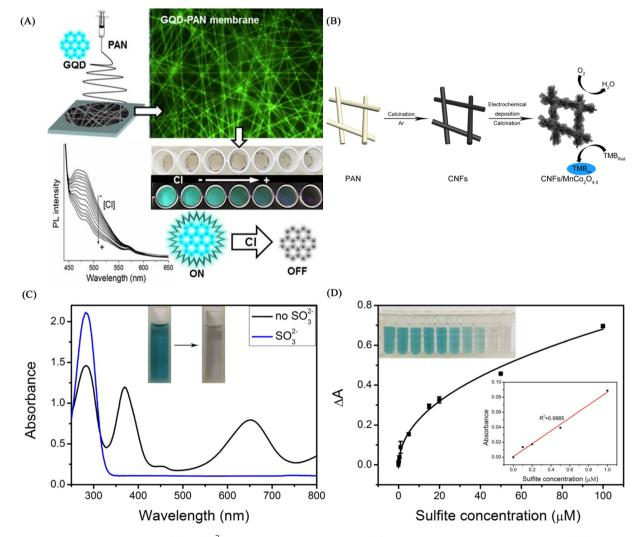
Fig. 21 Fabrication and properties of ClO<sup>-</sup>, So<sub>3</sub><sup>2</sup>-nanofiber membrane sensors (A) reprinted with permission from ref. 130. Copyright 2018, Elsevier. (B), (C) and (D) reprinted with permission from ref. 131. Copyright 2017, IOP Publishing Ltd.
