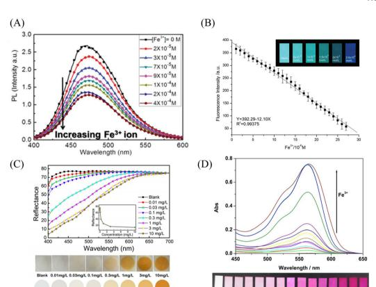
Fig. 10 Sensing properties of iron ion sensors preparted by chemical modification and copolymerization. (A) Reprinted with permission from ref. 102. Copyright 2015, *The Royal Society of Chemistry*. (B) Reprinted with permission from ref. 103. Copyright 2018, *Journal of The Brazilian Chemical Society*. (C) Reprinted with permission from ref. 104. Copyright 2019, *American Chemical Society*. (D) Reprinted with permission from ref. 105. Copyright 2015, Elsevier.
