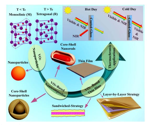
Scheme 1 Overview of VO<sub>2</sub>-based composites on durability against a harsh environment.
