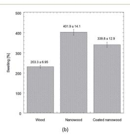
Fig. 5 (a) Plot comparing the water uptake on wood, nanowood and coated nanowood and (b) swelling percentage of each material after stability.
