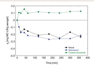
Fig. 6 Adsorption kinetic of wood, nanowood and the coated nanowood on a 5.4  $\mu g$  mL $^{-1}$  on a solution for 6 h.
