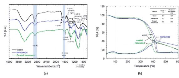
Fig. 3 (a) FTIR-ATR spectra of the wood, nanowood and coated nanowood and (b) shows the thermogravimetrical analysis of the three components with an insert table presenting the onset and max degradation temperatures of each one.
