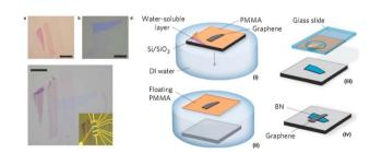
Fig. 2 Shows the mechanical stacking: a schematic depiction of the optical view, the transfer and stacking process of the graphene/h-BN devices (scale bars,  $10~\mu m$ ). Reprinted from ref. 61 by permission from Nature, copyright, 2010.
