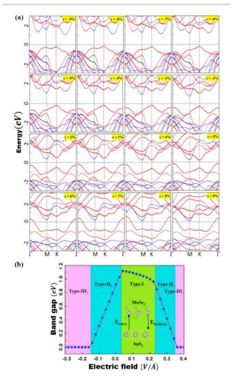
Fig. 9 (a) Under pressure, the band structures of MoSe<sub>2</sub>/SnS<sub>2</sub> heterojunctions. MoSe<sub>2</sub> and SnS<sub>2</sub> are represented by the red and blue lines, respectively. (b) The bandgap of MoSe<sub>2</sub>/SnS<sub>2</sub> heterojunctions varies as the external E-field changes. Reprinted from ref. 20 with permission from Elsevier, copyright 2021.
