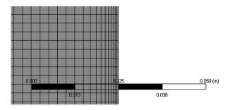
Fig. 3 Inflation method close up view
