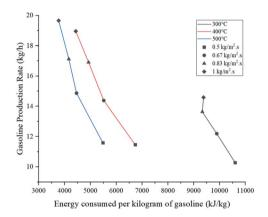
Fig. 10 Energy consumption at the operating conditions.
