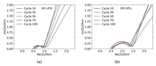
Fig. 4 Impedance spectra of Si electrodes cycled in (a) 1 M LiFSI and (b) 1 M LiPF<sub>6</sub>.
