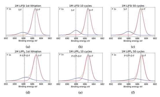
Fig. 8 F 1s spectra for Si electrodes cycled to 1st lithiation, cycle 10 and cycle 50 in LiFSI (a-c) respectively, and in LiPF<sub>6</sub> (d-f) respectively
