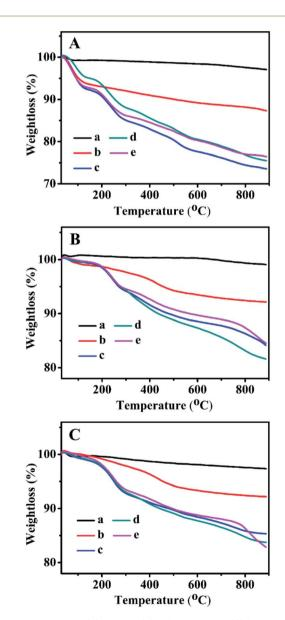
Fig. 6 TGA curves of (A) BMMs-, (B) MCM-41-, and (C) SBA-15-based samples. (a) Pure mesoporous materials, (b) Zn-modified samples, (c) Z1-immobilized samples, (d) Z2-immobilized samples, and (e) Z3-immobilized samples, in which the molar ratios of Z/Zn for all samples were around 1:1.
