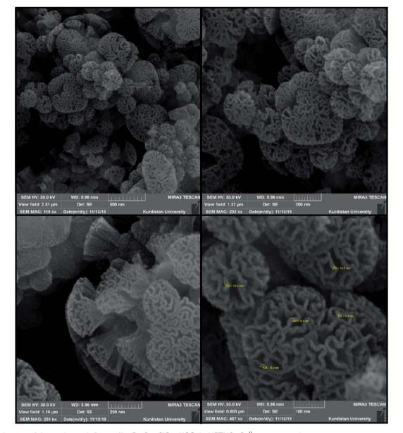
Fig. 4 SEM images of the cockscomb flower-like  $Fe_3O_4$ @Si $O_2$ @KCC-1@MPTMS@Cu $^{II}$  nanocomposite.
