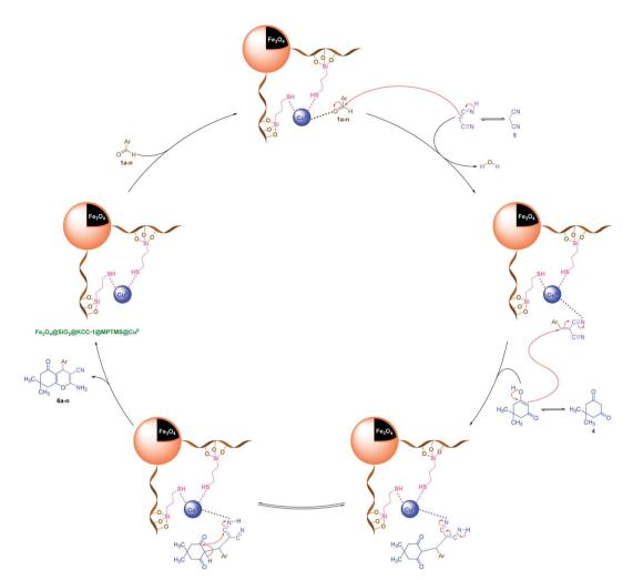
Scheme 6 Plausible mechanism for the solvent-free one-pot three-component synthesis of 2-amino-4-aryl-7,7-dimethyl-5-oxo-5,6,7,8-tetrahydro-4*H*-chromene-3-carbonitriles (6a–n) catalyzed by the Fe<sub>3</sub>O<sub>4</sub>@SiO<sub>2</sub>@KCC-1@MPTMS@Cu<sup>II</sup> nanocomposite.
