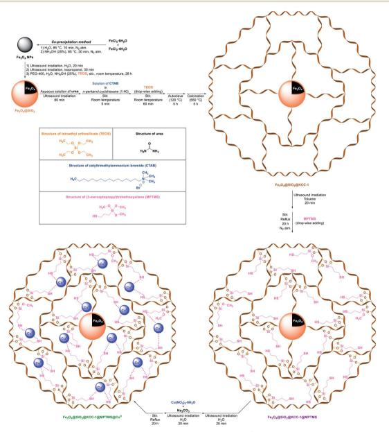
Scheme 1 Preparation of the cockscomb flower-like Fe<sub>3</sub>O<sub>4</sub>@SiO<sub>2</sub>@KCC-1@MPTMS@Cu<sup>II</sup> mesoporous nanocomposite.
