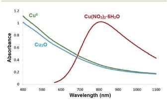
Fig. 9 UV-Vis spectra of the nanocomposite derived from the sources of  $Cu(NO_3)_2 \cdot 6H_2O$ ,  $Cu_2O$ , and  $Cu^0$ .
