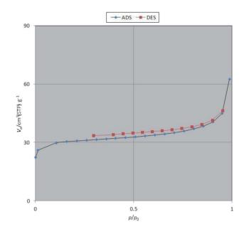
Fig. 10 Nitrogen ( $N_2$ ) gas adsorption—desorption profile of the asprepared Fe $_3O_4$ @Si $O_2$ @KCC-1@MPTMS@Cu $^{II}$  mesoporous nanocomposite.
