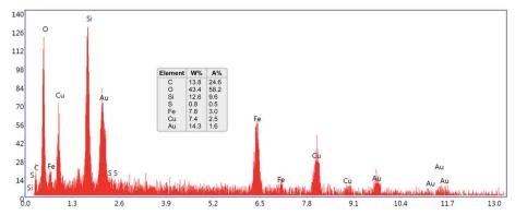
$\label{eq:Fig.6} \textbf{Fig. 6} \quad \text{SEM-based EDX spectrum of the } \text{Fe}_3\text{O}_4\text{@SiO}_2\text{@KCC-1@MPTMS@Cu}^{\text{II}} \text{ nanocomposite.}$
