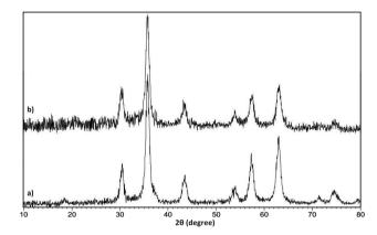
Fig. 3 PXRD patterns of the (a)  $Fe_3O_4$  and (b)  $Fe_3O_4$ @SiO $_2$ @KCC-1@MPTMS@Cu<sup>II</sup> nanostructures.
