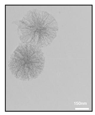
Fig. 12 TEM image of the recycled Fe $_3$ O $_4$ @SiO $_2$ @KCC-1@MPTMS@Cu $^{II}$  mesoporous nanocomposite.
