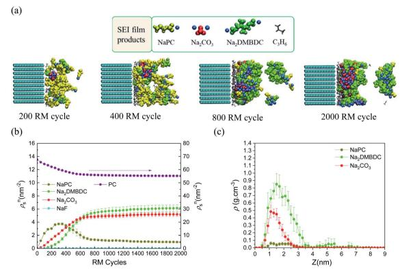
Fig. 2 (a) Typical snapshots of SEI layer formation during RM cycles in PC-based electrolyte solution. (b) Surface number densities  $(\rho_s^n)$  of SEI film products and solvent molecules,  $^{60}$  and (c) mass density distributions ( $\rho$ ) of SEI products.  $^{60}$  Copyright 2018, American Chemical Society.
