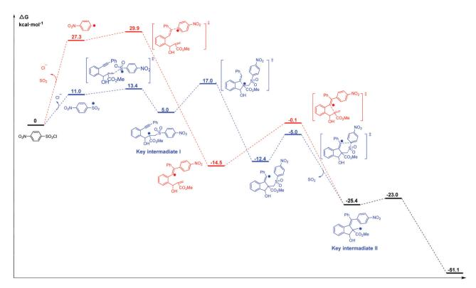
Fig. 9 Calculated free energy profiles for the two possible mechanisms (pathway proposed by Li et al. (red) and pathway proposed with the Transformer model (blue)),  $\Delta G$  values (in kcal mol<sup>-1</sup>) are calculated at 298 K.
