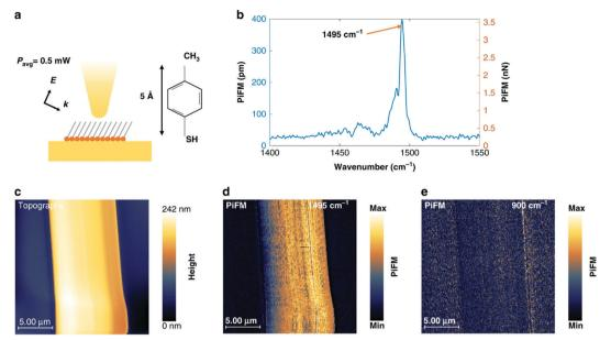
Fig. 1 Demonstration of monolayer response by PiFM. (a) 4-Methylbenzenethiol (4-MBT) adsorbed on template-stripped gold. Excitation average power is 0.5 mW focused to 20 μm-diameter spot. (b) Point spectrum of 4-MBT showing resonance at 1495 cm<sup>-1</sup>. (c) Topography of gold island. (d) PiFM image at 1495 cm<sup>-1</sup>. (e) PiFM image off resonance. (Reproduced from Almajhadi et al.<sup>32</sup>).
