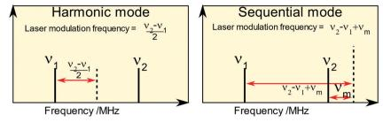
Fig. 17 Generalized heterodyne configurations proposed by Wang et al. 82 Harmonic heterodyne detection is illustrated for the first integer fraction of  $\nu_2 - \nu_1$ , but higher order fractions are also possible. Sequential mode involves the addition of another modulation which could be in intensity or for example in frequency.
