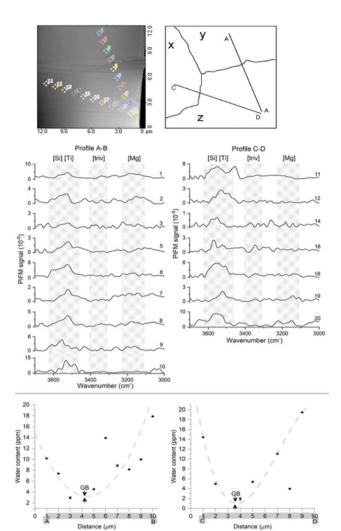
Fig. 12 Series of PiFM spectra from the polycrystalline forsterite sample. Two profiles are attained perpendicular to both two-grain boundaries. The water distribution profiles (bottom figure) were created using the estimated water content from point spectra. Patabendigedara et al. (Reproduced from Patabendigedara et al. 63).
