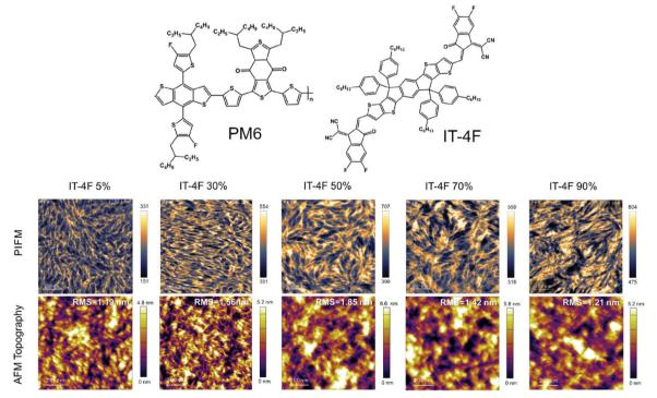
Fig. 3 Comparison of PiFM imaging of the distribution of IT-4F in PBDB-T-2F (PM6) using its IR absorption at 1288 cm<sup>-1</sup> with AFM imaging of the topography, (adapted from Fig. S4 of Mandemaker et al. 38).
