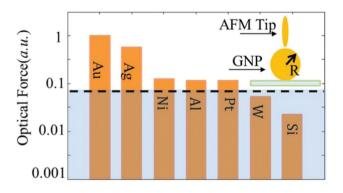
Fig. 19 Normalized optical force detected by AFM tips coated with different metals while measuring a 30 nm Au particle with incident light at 660 nm in the  $|E_z|$  incident field of different permittivity of the tip calculated by COMSOL. (Reproduced from Huang et al. 86).
