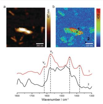
Fig. 5 PiFM maps at 1450 cm<sup>-1</sup> corresponding to the btc benzene breathing vibration, of a 1 layer HKUST-1 SURMOF thin film prepared using manual synthesis, including a drying step each half cycle. (b) Point IR spectra taken at positions 1 (red) and 2 (black), on and off the top of a high feature. (Reprinted from Delen et al.41).
