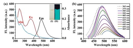
Fig. 5 (a) UV absorption spectrum and emission spectrum of the m-Q[6]-CQDs. The illustrations are the optical images of m-Q[6]-CQDs solution (i) under natural light irradiation and (ii) ultraviolet lamp irradiation; (b) fluorescence emission spectra of m-Q[6]-CQDs at excitation wavelengths of 365– 465. The solvent used is ultrapure water.
