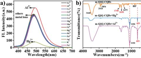
Fig. 7 (a) Interaction of the m-Q[6]-CQDs with different metal ions under neutral conditions, the m-Q[6]-CQDs concentration is 0.38 mg mL<sup>-1</sup>,  $\lambda_{\rm ev}/\lambda_{\rm em}$  = 385/485 nm; (b) comparison of the infrared spectra of the m-Q[6]-CQDs with Hg<sup>2+</sup> and Al<sup>3+</sup>. The concentration of all metal ions is 0.2 mM. The solvent used is ultrapure water.
