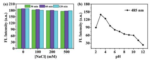
Fig. 6 (a) The effect of ionic strength on the fluorescence intensity of the m-Q[6]-CQDs; (b) the effect of pH on the fluorescence intensity of the m-Q[6]-CQDs; the m-Q[6]-CQDs concentration was 0.1 mg mL<sup>-1</sup>,  $\lambda_{ex}/\lambda_{em}$  = 385/485 nm. The solvent used is ultrapure water.
