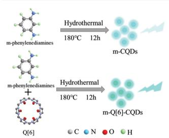
Fig. 1 Preparation of m-CQDs and m-Q[6]-CQDs
