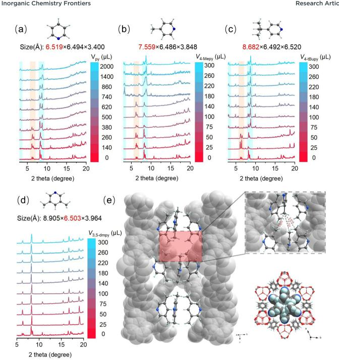
Fig. 1 Geometry-quided synthesis of MIL-101(Mn) through introducing geometrical modulators such as (a) pyridine, (b) 4-methylpyridine, (c) 4-tertbutylpyridine and (d) 3,5-dimethylpyridine, tested by PXRD. (e) Overall and detailed structure of the unexpected MIL-88B(Mn) phase, showing the channel alone c-axis. Note that the red and blue regions highlighted in (a)-(c) correspond to the characteristic peaks of MIL-88B(Mn) and MIL-101(Mn) phases, respectively.
