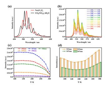
Fig. 30 (a) Solid-state photoluminescence emission spectra of Na@U<sub>6</sub>P<sub>6</sub> and UO<sub>2</sub>(NO<sub>3</sub>)<sub>2</sub>·6H<sub>2</sub>O ( $\lambda_{ex}$  = 441 nm, normalized intensity); (b) emission map of spectra recorded from 100 to 300 K; variation trend of emission peaks depends on temperature for (c) Na@U6P6 and (d) U3. Reprinted with permission from ref. 41 and 62. Copyright 2021 American Chemical Society and 2022 Elsevier, respectively.
