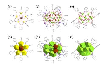
Fig. 21 Views of (a and b)  $[U(UO_2)_5(\mu_3-O)_5(PhCOO)_5(Py)_7]$ , (c and d) {[K  $(Py)_2]_2[K(Py)]_2[U_{16}O_{24}(PhCOO)_{24}(Py)_2]$ }, (e and f)  $[U_{10}O_8(OH)_6(PhCO_2)_{14}I_4(H_2O)_2(MeCN)_2]$ . Color codes:  $U^{IV}$ , green;  $U^V$ , brown;  $U^{VI}$ , yellow; I, violet. Other color codes are the same as in Fig. 1.
