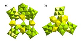
Fig. 28 Views of (a)  $[((UO_2)(H_2O))_3Nb_{46}(UO_2)_2O_{136}H_8(H_2O)_4]^{24-}$  and (b)  $[(Nb_7O_{22}H_2)_4(UO_2)_7(H_2O)_6]^{22-}$ . Color codes are the same as in Fig. 1; Nb,
