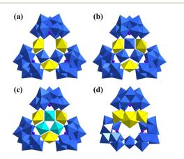
Fig. 8 Views of (a)  $[(UO_2)_3(H_2O)_5As_3W_{29}O_{104}]^{19-}$ , (b)  $[(UO_2)_3(H_2O)_6As_3W_{30}O_{105}]^{15-}$ , (c)  $[(UO_2)_3(H_2O)_6As_3W_{29}V^{IV}O_{105}]^{17-}$ , and (d)  $[(UO_2)_3(H_2O)_4As_3W_{26}O_{94}]^{17-}$ . Color codes are the same as in Fig. 1.
