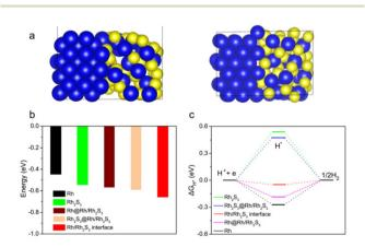
Fig. 7 DFT calculation of the HER process on p-Rh/Fe-Ni<sub>3</sub>S<sub>2</sub>/NF. (a) Side (left) and top view (right) of the model surface used for the Rh<sub>2</sub>S<sub>3</sub>/ Rh heterointerface. Blue and yellow balls represent Rh and S atoms, respectively; calculated water adsorption energies (b) and  $\Delta G_{H^*}$  (c) on Rh<sub>2</sub>S<sub>3</sub>/Rh, Rh<sub>2</sub>S<sub>3</sub> and Rh.
