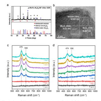
Fig. 4 Post-OER characterization of p-Rh/Fe-Ni<sub>3</sub>S<sub>2</sub>/NF after 50 h of the OER at 100 mA cm $^{-2}$ : (a) XRD pattern and (b) TEM images. (c and d) OER in situ Raman spectra of (c) p-Rh/Fe-Ni<sub>3</sub>S<sub>2</sub>/NF and (d) Fe-Ni<sub>3</sub>S<sub>2</sub>/NF at different polarized potentials.
