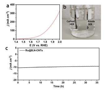
Fig. 6 (a) The LSV curve for the assembled electrolyzer in 1 M KOH employing Ru@B,N-CNT electrocatalysts as both anode and cathode. (b) A photograph of the assembled electrolyzer using Ru@B,N-CNTs as both cathode and anode. (c) The chronoamperometric i-t curve measured at an applied potential of 1.57 V for the electrolyzer assembled with Ru@B,N-CNT electrocatalysts for 36 h.
