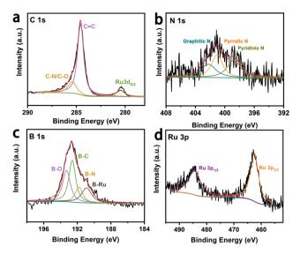
Fig. 2 High resolution XPS for (a) C 1s, (b) N 1s, (c) B 1s, and (d) Ru 3p of the Ru@B,N-CNTs.
