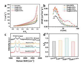
Fig. 3 (a) The  $N_2$  sorption isotherms, (b) the corresponding pore size distributions, (c) the Raman spectra, and (d) the corresponding  $I_D/I_G$ ratios, of the B,N-CNTs, Ru@B,-CNTs, Ru@N-CNTs and Ru@B,N-CNTs.
