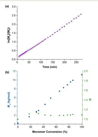
Fig. 4 Polymerization of 1c with Ru-1 ([1c]: [Ru-1] = 50:1): (a) Determination of the rate of propagation ( $R^2 = 0.998$ ) at 32 °C in  $CD_2Cl_2$ ; (b)  $M_n$  (blue squares) and  $\mathcal{D}$  (green triangles) vs conversion.
