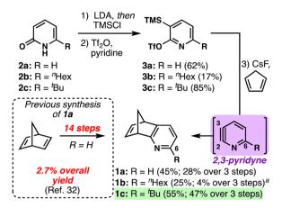
Fig. 2 Synthesis of pyridinonorbornenes 1a-c via 2,3-pyridynes. Reagents and conditions: (1) LDA (2.2 equiv.), THF, 0 °C, 1 h, then TMSCl (1.2 equiv.), 0 °C, 15 min, then rt, 12 h. (2) Tf<sub>2</sub>O (1.1 equiv.), pyridine, 0 °C, 20 min, then rt, 12 h. (3) CsF (5.0 equiv.), C<sub>5</sub>H<sub>6</sub> (5.0 equiv.), MeCN, 30 °C, 3 h. a4 : 1 MeCN : DCM.
