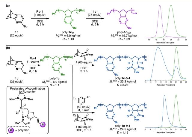
Fig. 5 (a) Synthesis of poly-1c<sub>100</sub> via chain extension. (b) Synthesis of diblock copolymer poly-1c-b-4 using 3-bromopyridine to facilitate reinitiation of the chain ends.
