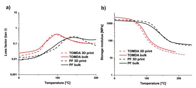
Fig. 12 (a) Loss factor of bulk cured and 3D printed parts. (b) Storage modulus G' curves of bulk cured and 3D printed parts.
