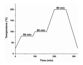
Fig. 1 Post-processing program with a heating rate of 2 K min<sup>-1</sup>.
