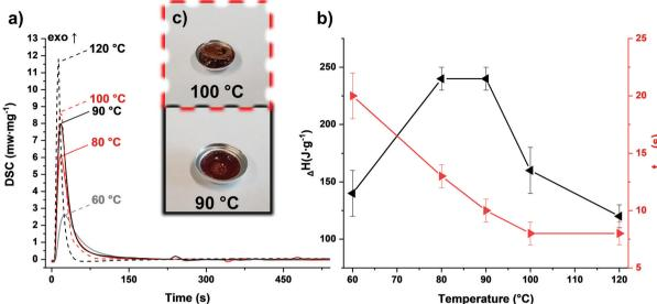
Fig. 3 (a) Photo-DSC of the PF-formulation at 60-120 °C,  $2 \times 900$  s, 320-500 nm, 60 mW cm<sup>-2</sup>. (b) Temperature dependence of photo-DSC results for the PF-formulation: enthalpy change ( $\Delta H$  black) and time until maximal heat is released ( $t_{max}$  red). (c) Cured Samples at 90 & 100 °C.
