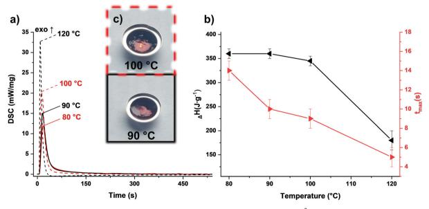
Fig. 5 (a) Photo-DSC of the TOMDA-formulation at 80-120 °C,  $2 \times 900$  s, 320-500 nm, 60 mW cm<sup>-2</sup>. (b) Temperature dependence of photo-DSC results for the TOMDA-formulation: enthalpy change ( $\Delta H$  black) and time until maximal heat is released ( $t_{max}$  red). (c) Cured Samples at 90 & 100 °C.
