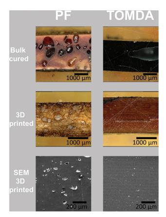
Fig. 10 Microscopic images of the different produced specimen after post-curing
