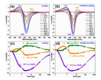
Fig. 6 Femtosecond transient absorption (fs-TA) spectra of (a) CsPbBr $_3$ , (b) CsPbBr $_3$ /Cs $_4$ PbBr $_6$  measured for various pump-probe delay times at 400 nm excitation, excited-state kinetic curves for the PA1, GSB, and PA2 of (c) CsPbBr $_3$ , (d) CsPbBr $_3$ /Cs $_4$ PbBr $_6$ .
