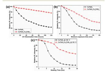
Fig. 8 (a) UV irradiation test, (b) moisture resistance test, and (c) thermal tolerance test for CsPbBr3 NCs and dual-phase CsPbBr3/ Cs<sub>4</sub>PbBr<sub>6</sub> MCs conducted by monitoring their emission trends at 365 nm excitation.
