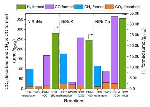
Fig. 4 Results of feasibility study of flexible DFMs, showing the amount of CO<sub>2</sub> desorbed and products formation in each reaction for NiRuNa, NiRuK and NiRuCa.
