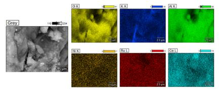
Fig. 12 SEM and EDX mapping of NiRuk.
