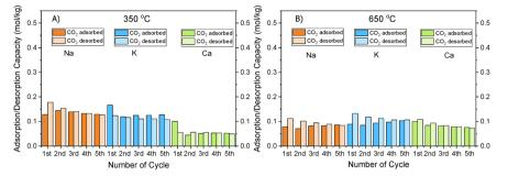
Fig. 3 CO<sub>2</sub> Adsorption/desorption cycles of Na, K and Ca at (A) 350 °C and (B) 650 °C.
