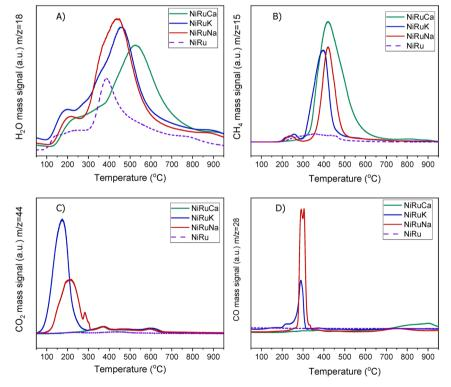
Fig. 5 H<sub>2</sub>-TPR study for NiRuNa, NiRuK, NiRuCa and NiRu: (A) H<sub>2</sub>O, (B) CH<sub>4</sub>, (C) CO<sub>2</sub> and (D) CO signals.
