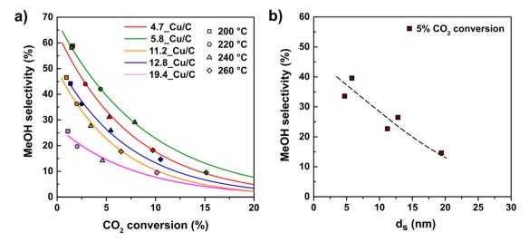
Fig. 5 (a) MeOH selectivity as a function of CO<sub>2</sub> conversion for catalysts with different Cu particle sizes. (b) Selectivity to MeOH as a function of Cu particle size for a CO<sub>2</sub> conversion of ~5%. The trend line was added to guide the eye. Reaction conditions: 4.2 mg of Cu per reactor, 40 bar(g), 600 mL min<sup>-1</sup>  $g_{Cu}^{-1}$ ,  $H_2/CO_2/He = 67.5/22.5/10$  vol%.
