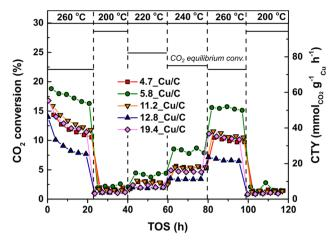
Fig. 3 Characteristic profiles for CO<sub>2</sub> conversion and weight-normalized copper time yield for Cu/C catalysts as function of TOS (h) at different temperatures. Reaction conditions: 4.2 mg of Cu per reactor, 40 bar(g), 600 mL min<sup>-1</sup>  $g_{Cu}^{-1}$ ,  $H_2/CO_2/He = 67.5/22.5/10 vol%.$
