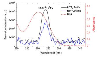
Fig. 4 UVC UCL emission spectra of LiYF<sub>4</sub>:Pr<sup>3+</sup>/Yb<sup>3+</sup> NC powder (black solid line) and NaYF<sub>4</sub>:Pr<sup>3+</sup>/Yb<sup>3+</sup> NCs (blue solid line) with 10 mol% Yb<sup>3+</sup> concentration under 447 nm laser excitation and comparison with the DNA absorption spectrum (red dotted line).
