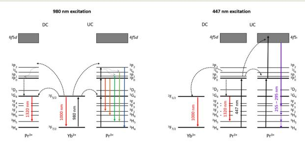
Fig. 1 A scheme of electronic levels and transitions corresponding to VIS-to-UVC UCL and NIR-to-NIR-II DCL processes in Pr3+ and Yb3+ in fluoride NCs. The UCL and DCL mechanisms are illustrated under (a) 980 nm laser excitation for visible and NIR emissions and (b) 447 nm laser excitation for UVC and NIR emissions.
