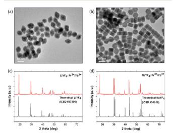
Fig. 2 Selected TEM images of (a) LiYF<sub>4</sub>:Pr $^{3+}$ /Yb $^{3+}$  and (b) NaYF<sub>4</sub>:Pr $^{3+}$ / Yb3+ NCs. The corresponding PXRD patterns of (c) LiYF4:Pr3+/Yb3+ and (d) NaYF<sub>4</sub>:Pr<sup>3+</sup>/Yb<sup>3+</sup> NCs versus theoretical patterns from the database.
