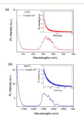
Fig. 5 NIR-II PL spectra of LiYF<sub>4</sub>:Pr<sup>3+</sup>/Yb<sup>3+</sup> (a) and NaYF<sub>4</sub>:Pr<sup>3+</sup>/Yb<sup>3+</sup> (b) NCs in CHCl3. Insets of a and b show corresponding DCL decays acquired at 1320 nm under 980 nm excitation.
